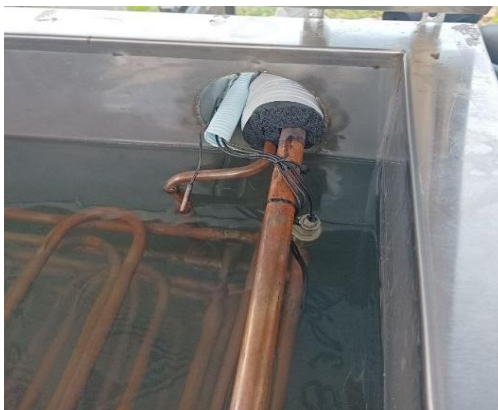
Figure 22. Heat exchanger of the cooling system (a) and sensor for controlling water temperature (b)
