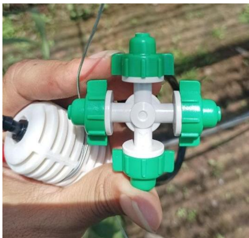
Figure 18. Fogger of the spraying system
