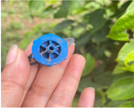
Figure 36. Emitter for drip irrigation system at Reksa Farm
